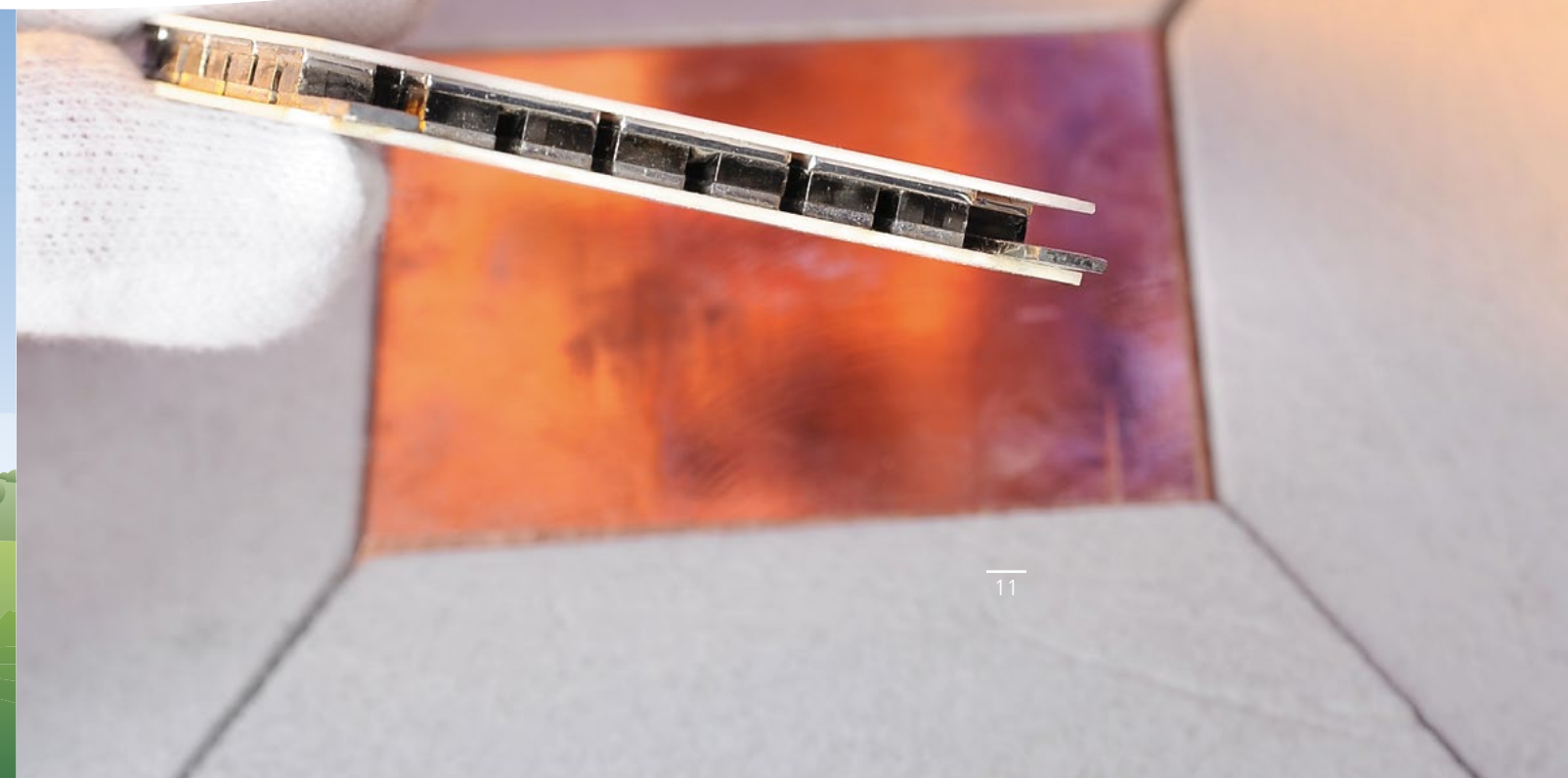
Electrical power from heat – thermoelectric generator module
