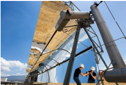
Mirrors under test – quality investigations at the Plataforma Solar in Almería (southern Spain)
